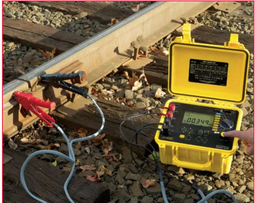
Verifying rail bonds with the Model 6250
